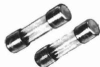
These time lag glass fuse links have a better than normal, reliable anti-surge property. They are used for the protection of telecommunication and electrical equipment. They comply with BS4265, CEE4 and IEC127 standard sheet III.
