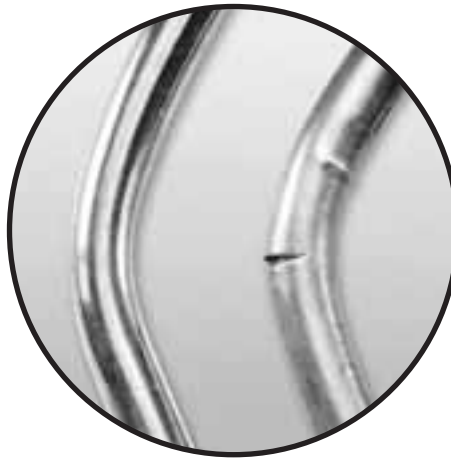
Figure 11. Photo shows two ground rods subjected to the same pressure load test. The ERITECH® copperbonded ground rod, shown on the left, will bend without tears, cracks or folds, to the outer sheath. The inferior copperclad rod shown on right, has developed cracks and creases to the outer sheath, which will significantly reduce its servicable life and put the integrity of the entire electrode at risk.
