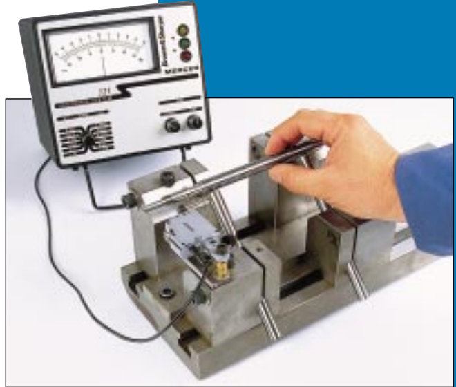
Drunkness checker measures deviation within one turn.
