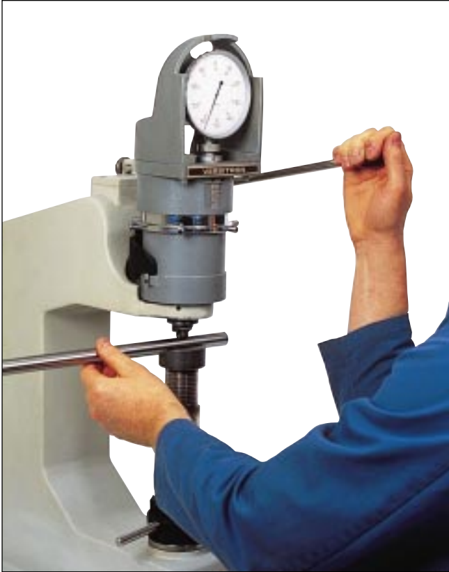
Lead screw hardness test using a Rockwell Hardness Tester. Maintains material quality and 100% reliability.
