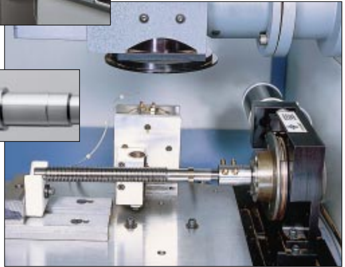
Serial number, lead, and accuracy etched into lead screw and nut with a Laser Marking Machine.
