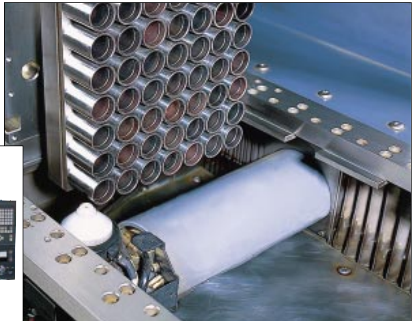
Cutting a pallet of thrust bushings using Electrical Discharge Machining (EDM).
