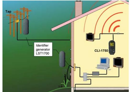
Home leakage detection configuration using the LST-1700 as a signal identifier.
