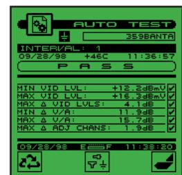
Auto Test results are time, date, and temperature stamped and can be stored, viewed, printed, or uploaded to JDSU’s StealthWare software.
