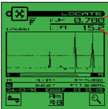
VOP is entered on the keypad or calculated with a known length of cable.
