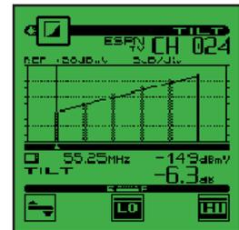
The tilt display shows six channels and updates in less than a second.
