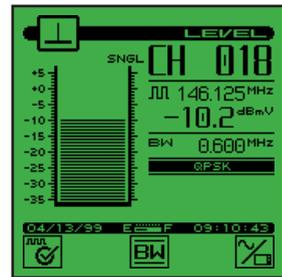
“Small-band” digital carriers, like cable telephony, require a different measurement technique. For that purpose, the digiCheck feature offers a time average as well. Even in this case, all level readings are fully compensated for by the correct occupied bandwidth.
