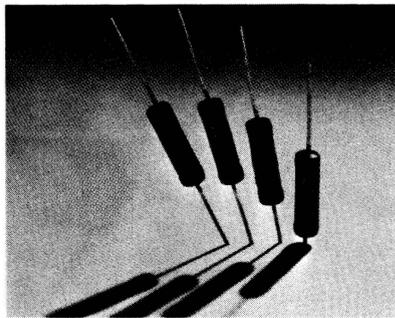
These resistors have a permissible hot-spot temperature of 400 °C. The leads are of a special material with high thermal resistance to counter temperature effects of the solder joint. The coating is a high quality vitreous enamel.
