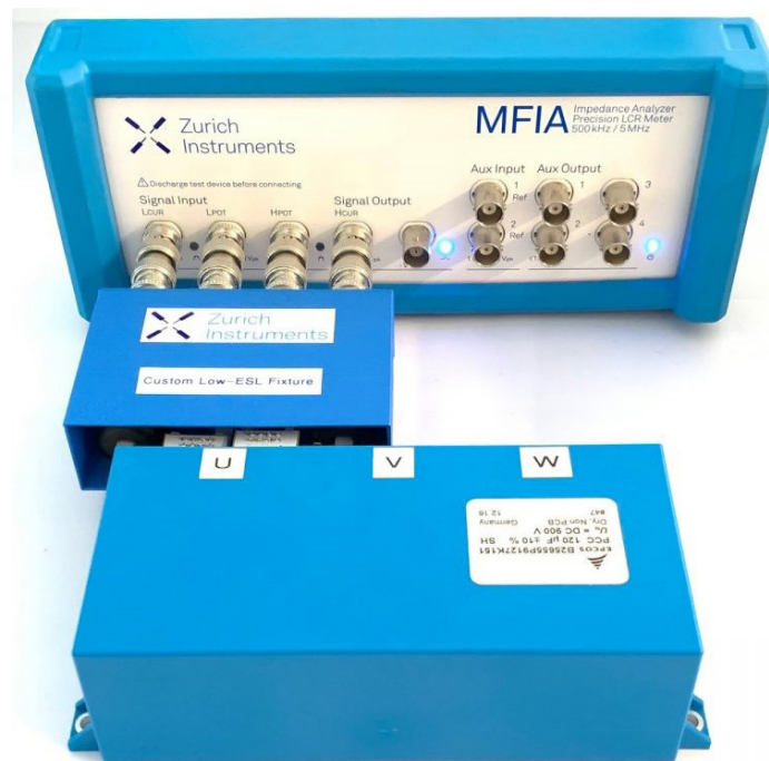
Figure 3: Test setup for measuring the ESL and ESR of a DC-Link capacitor. Source: Zurich Instruments
