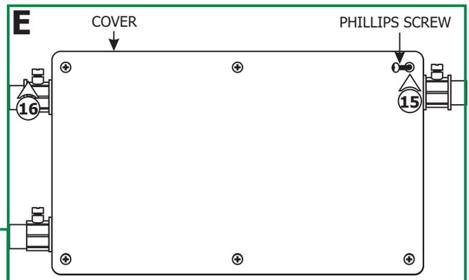
**15:** Replace the power supply cover and secure it by tightening the six Phillips screws.
