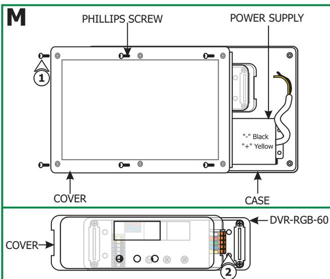
**NOTE:** Refer to the instructions provided with the CDP (Color Dial Controller) or CTP (Color Touch Screen Controller) to install, power, and program them. This section shows typical CDP controller installation.
