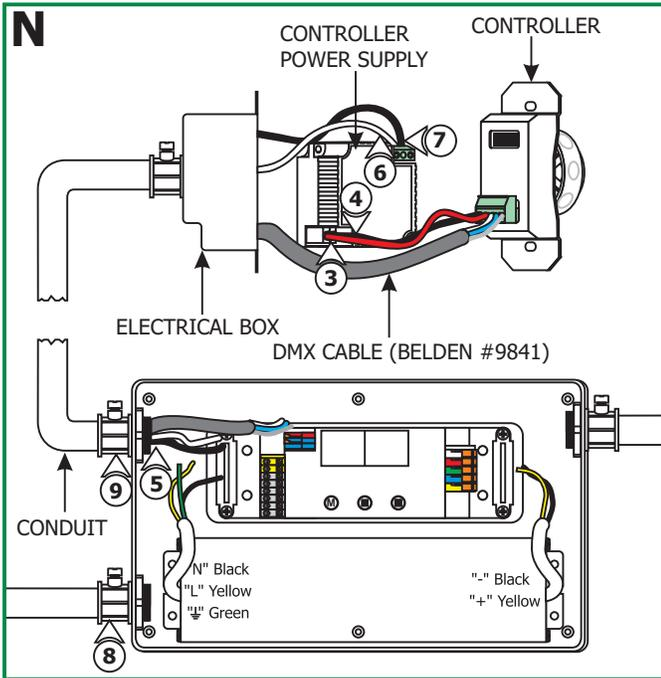
**NOTE:** Use a deep double gang boxes to fit the controller and controller power supply (OT-20-120-240-245 recommended).
