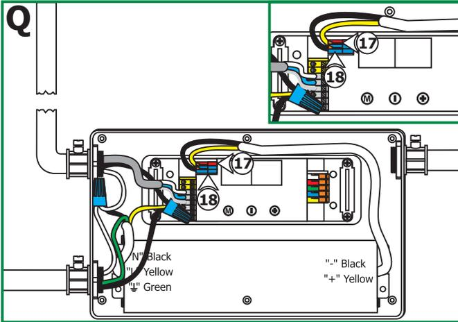
**17:** Connect the yellow power supply wire marked "+" to DVR-RGB-60 "Vdc+" red terminal.
