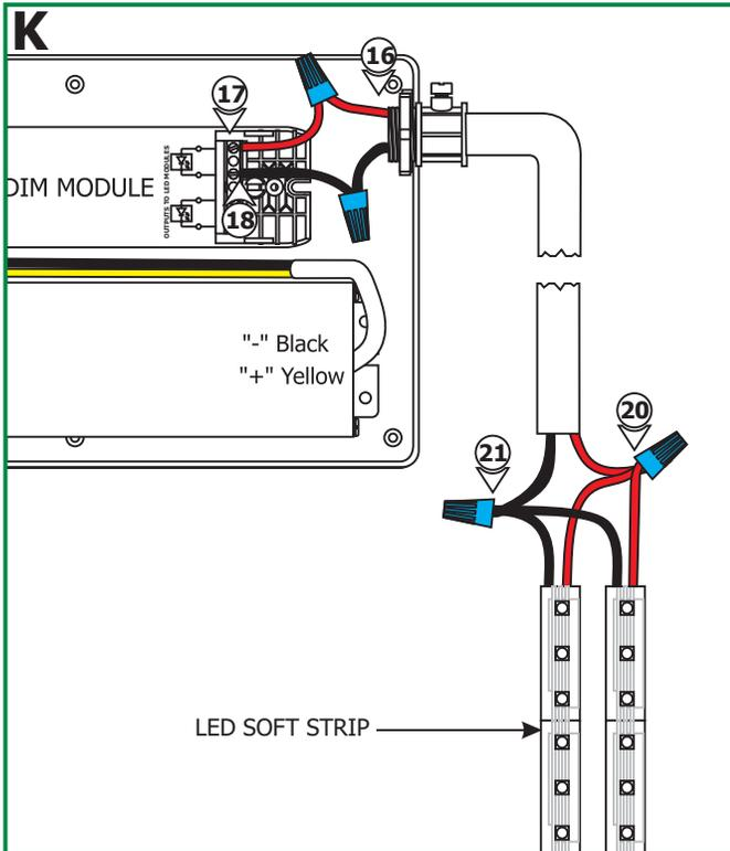
**15:** Use the "Low Voltage Wire Size Chart" on page 1 to determine the proper wire size connecting the dim module to the LED soft strip.
