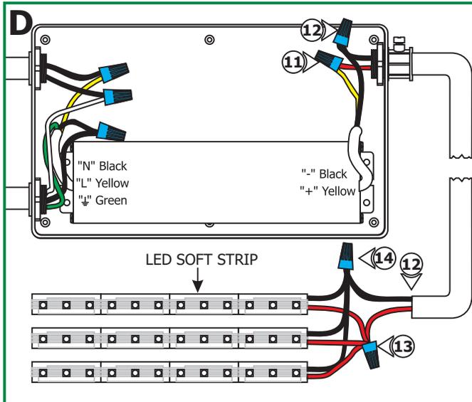
**9:** Use the "Low Voltage Wire Size Chart" on page 1 to determine the proper wire size connecting the power supply to the LED soft strip.
