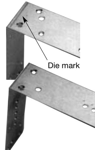
Most European-style punches come with a variety of tip radii. To form mild and stainless steels, select a punch-tip radius roughly half the material thickness being formed. Since the V opening will determine the formed inside bend radius, punch-tip radius should not exceed the material thickness, or else the inside bend radius will increase. When
