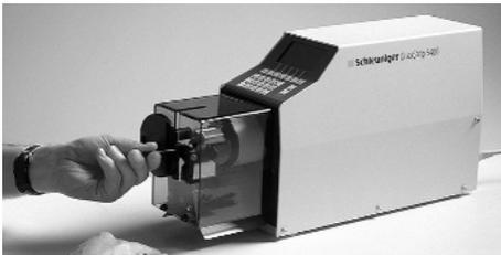
**Sensor Activated Start Cycle:** Some machines require a button or a footpedal to be depressed to activate the machine cycle. Others use a sensor that detects the cable end to begin the machine cycle. The "sensor type" is preferred by most operators because it requires one less operation compared to pressing a button or a footpedal. If it is a sensor type, verify that even your smallest cable can trigger it without the cable buckling.
